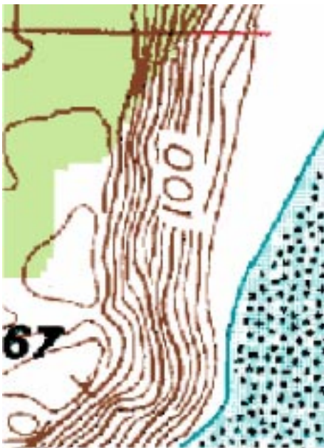
Topographic map of seacliff area used in these illustrations. 20 foot contours and 111 meters (367 feet) of relief.
