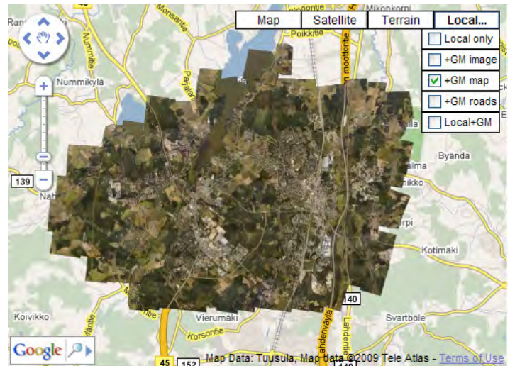
Google Maps custom map (mashup) with local Tuusula, Finland orthoimage Tile Overlay on top of Google's map. The sample HTML file created with the Tile Overlay in the TNTmips Mosaic process sets up a Local menu button with a series of custom map choices that show various combinations of the local Tile Overlay and Google's map and image layers.
