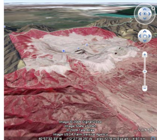
Perspective view in Google Earth of the Super-Overlay created from the small mosaic layout shown on this page. Google's Super-Overlay tileset structure provides the fastest possible display of your very large overlays in Google Earth.
